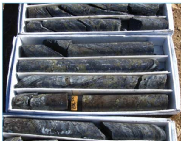
Figure 7-6: Manto Replacement Mineralization After Limestone
