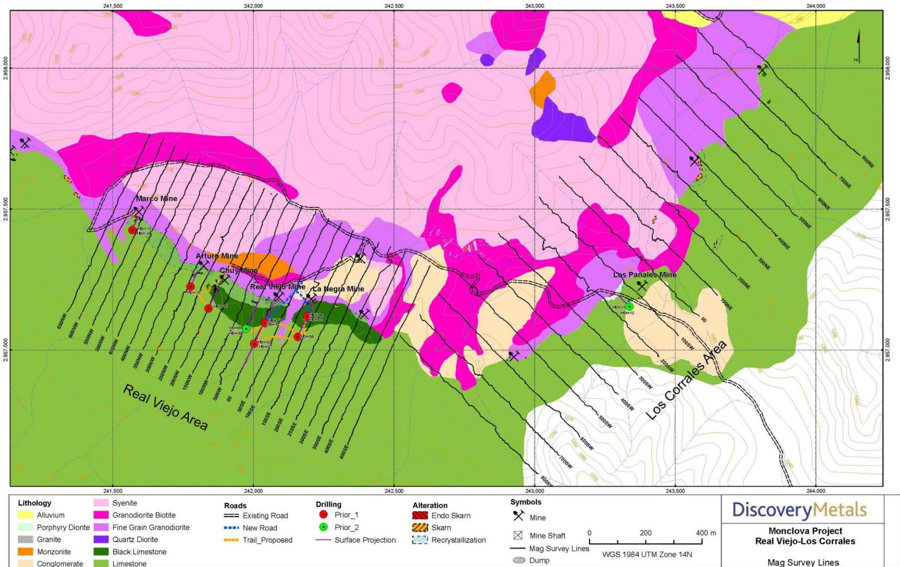
Fig. 41. Geologic map of the Real Viejo and Los Corrales areas with the lines of the ground magnetometer survey.
