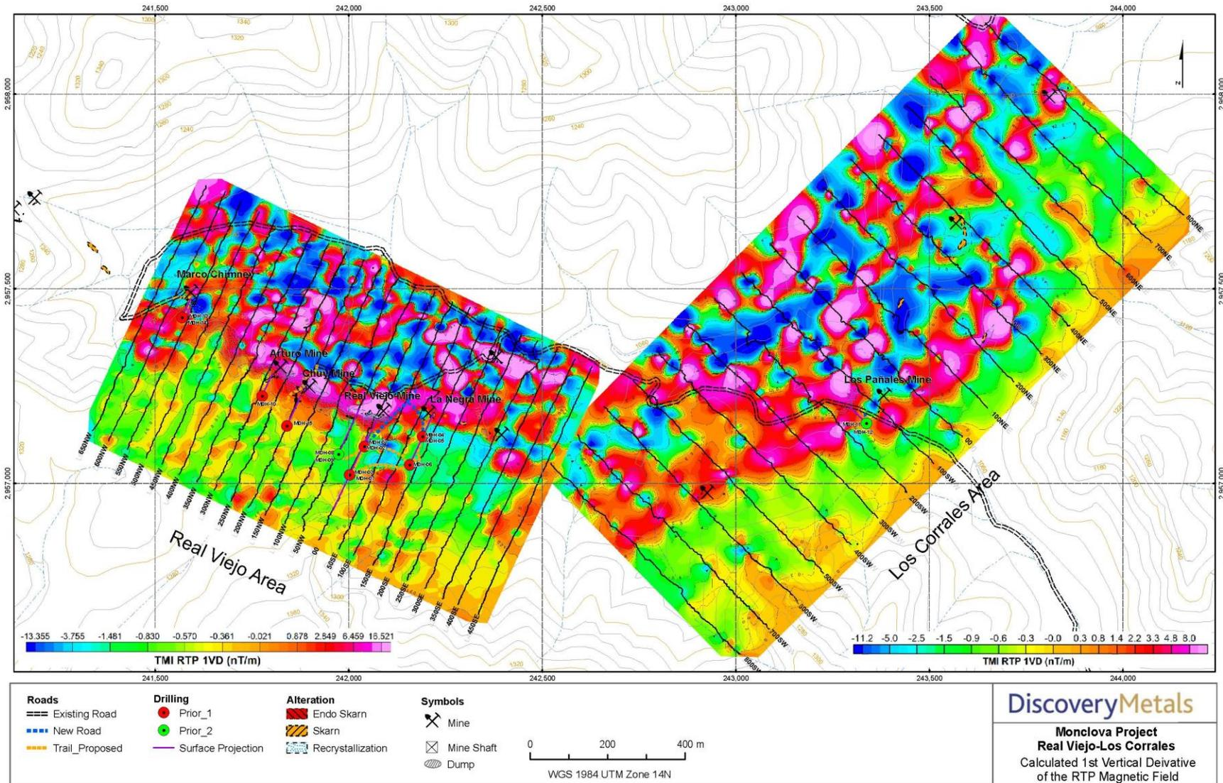
Fig. 43. Results of the ground magnetometer survey for the Real Viejo and Los Corrales areas showing the first vertical derivative of the reduced to the pole magnetic data. Several anomalies are indicated. Planned drill holes from DSV.
