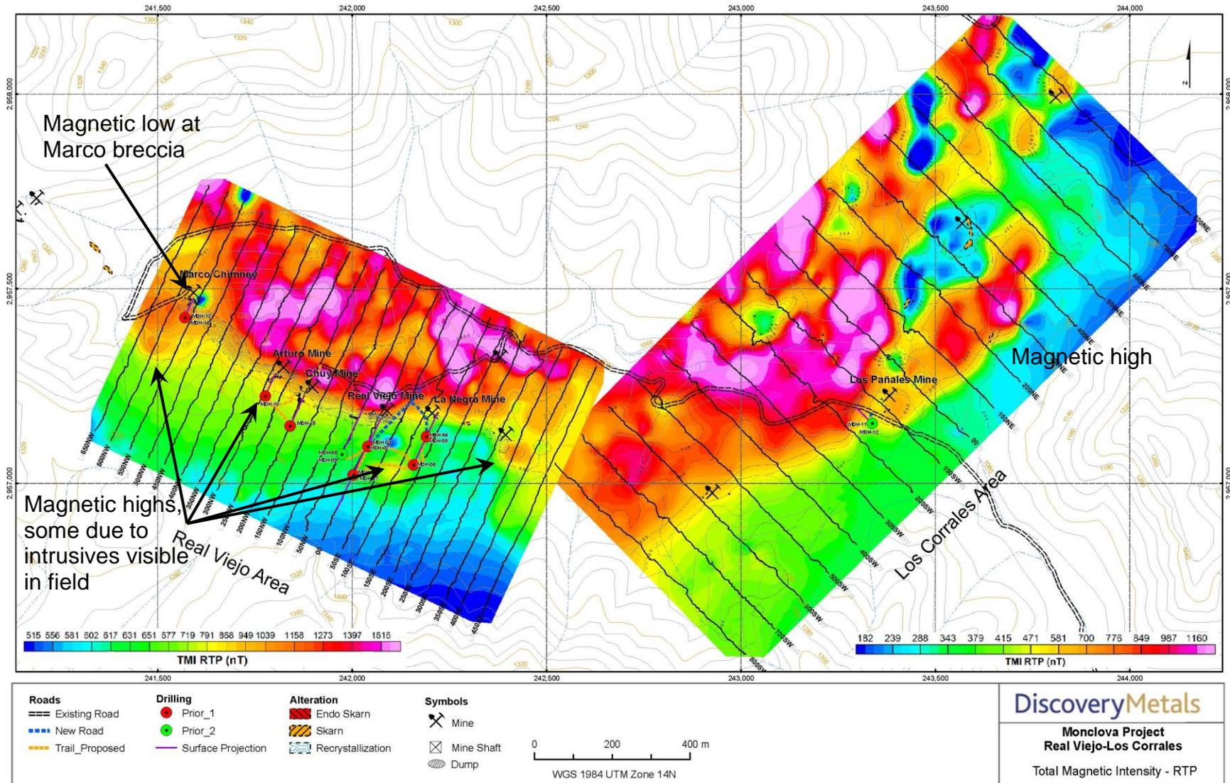
Fig. 42. Results of the ground magnetometer survey for the Real Viejo and Los Corrales areas showing total magnetic intensity, reduced to the pole. Several anomalies are indicated. Planned drill holes from DSV.
