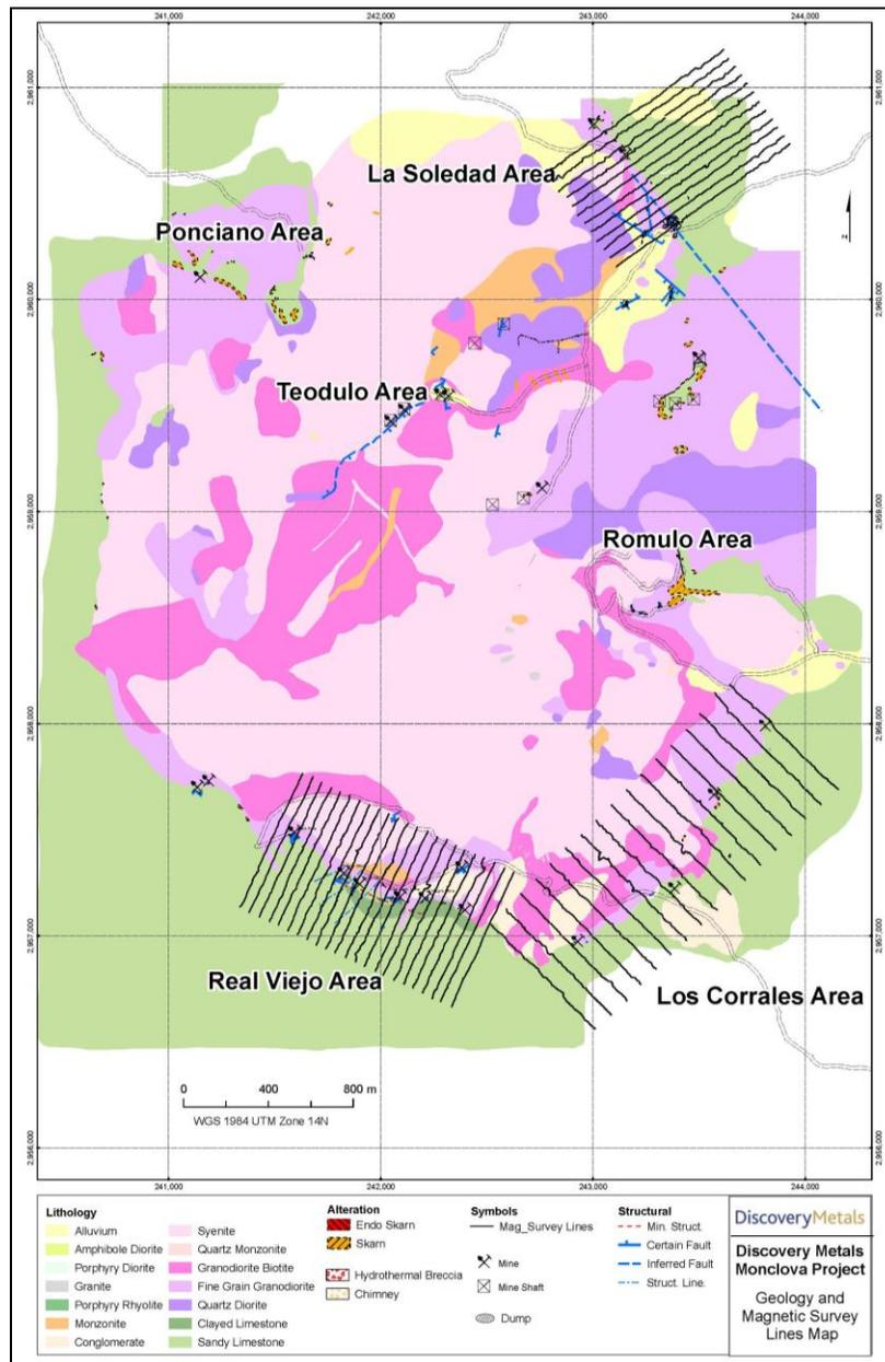
Fig. 37. Geologic map with ground magnetic grid lines for the Monclova project.
