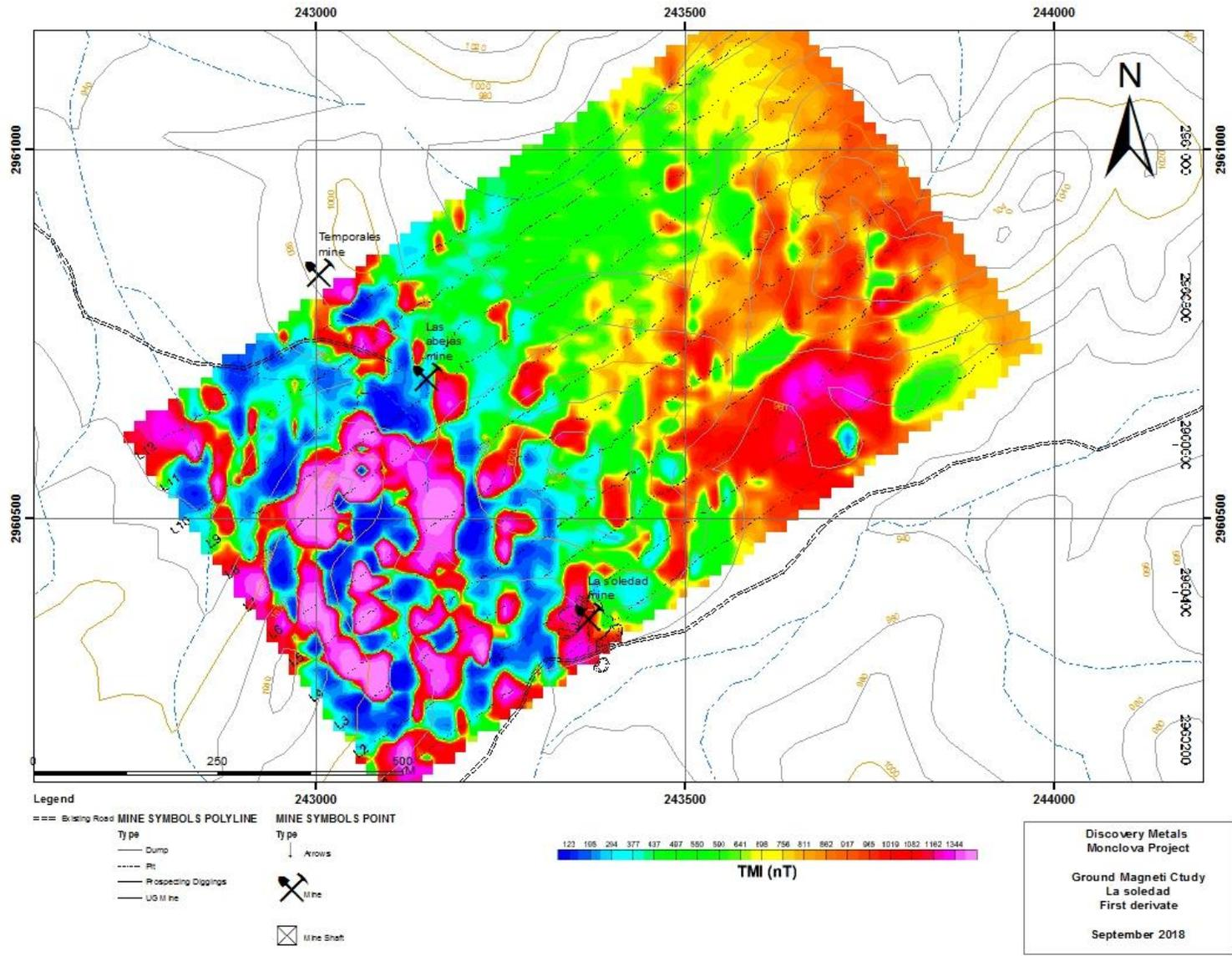
Fig. 40. Results of the ground magnetometer survey for the Soledad area showing the first vertical derivative of RTP.
