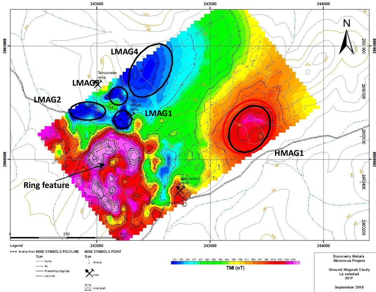
Fig. 39. Results of the ground magnetometer survey for the Soledad area showing total magnetic intensity, reduced to the pole (RTP). Several magnetic lows and highs are present.
