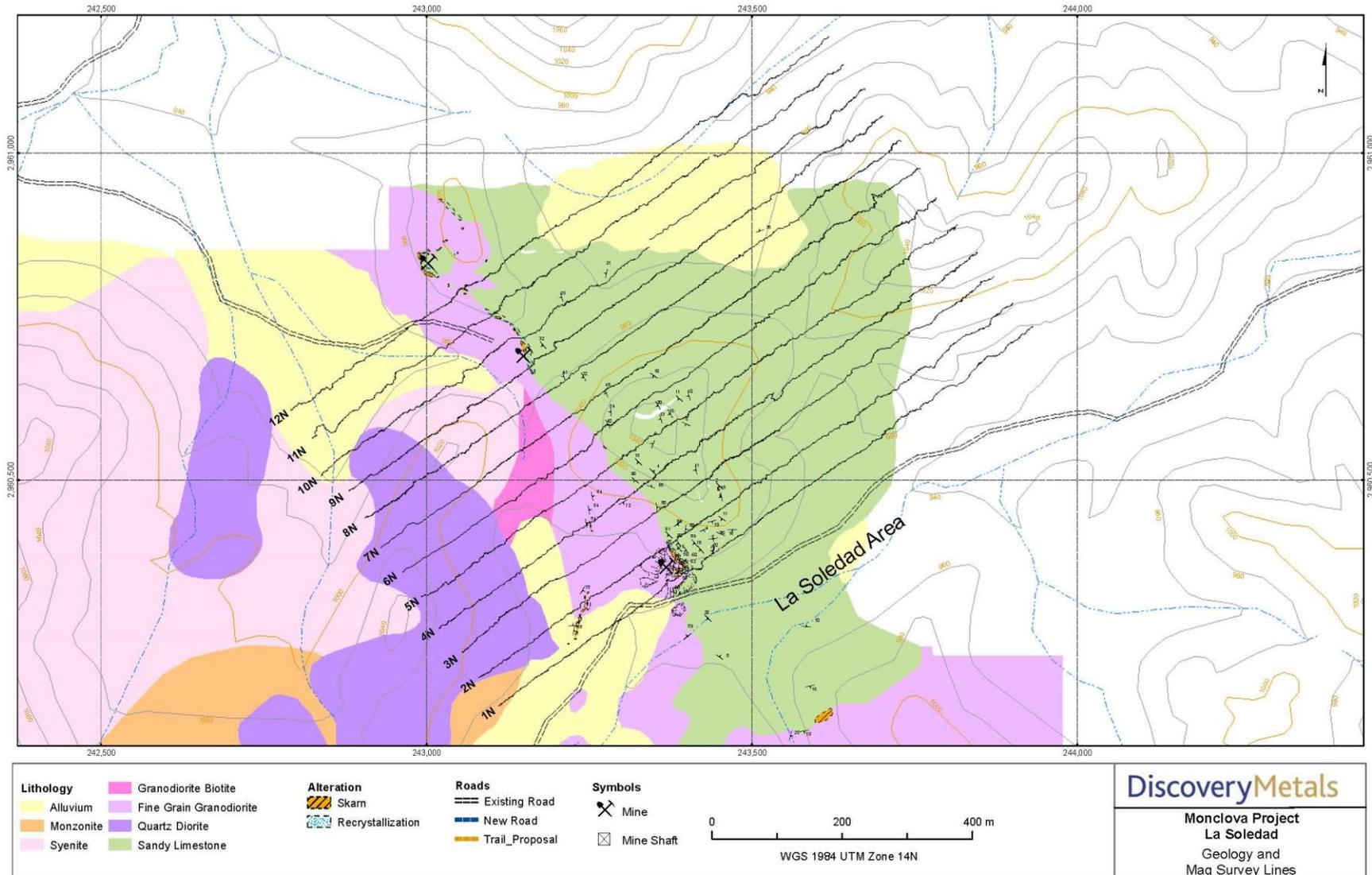
Fig. 38. Geologic map of the Soledad area with the lines of the ground magnetometer survey.
